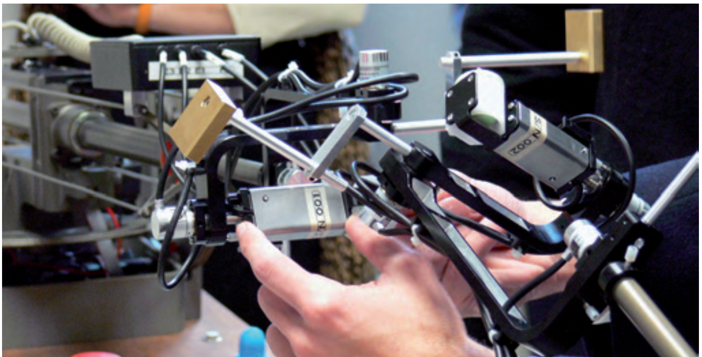
Fingers are inserted into the device, through which touch stimuli provide information about the contact being made with the object
