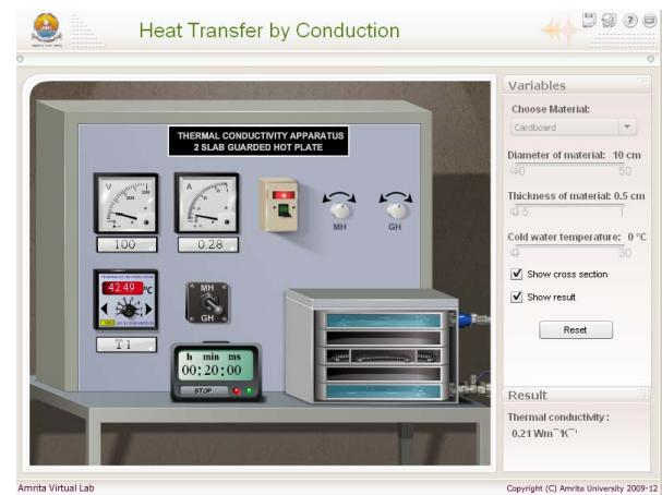
Figure 2: Simulation of Heat Conduction Apparatus
