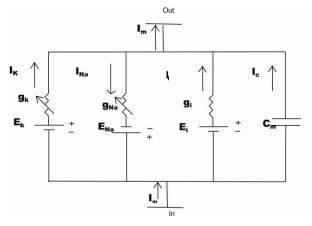
Figure 2: Neural equivalent circuit
