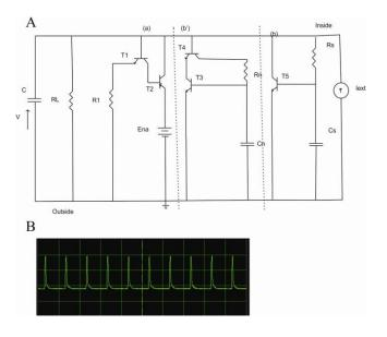
Figure 14: Hardware neuron with periodic bursting.
