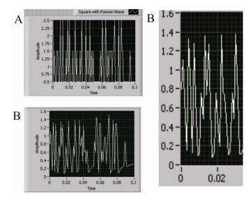
Figure 11: A represent input excitation with Poisson noise. B the corresponding noise and C represent single spike enlarged.
