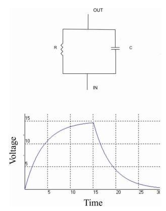
Figure 1: RC circuit and output wave form.
