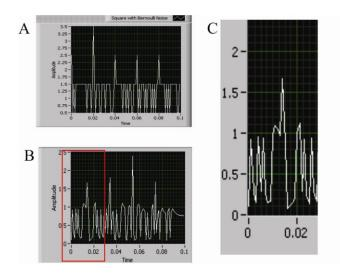
Figure 12: A input excitation with Bernoulli noise; B shows noisy output; C zoomed output.
