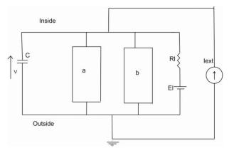
Figure 4: Equivalent circuit of HH neuron proposed by Hoshimiya [7]
