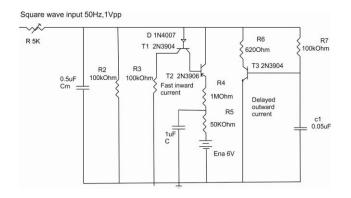
Figure 7: Analog neuron model with ionic channels.
