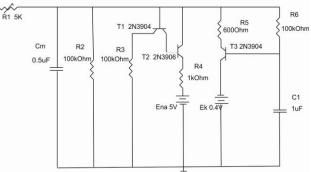
Figure 6: Simple analog neuron model circuit.
