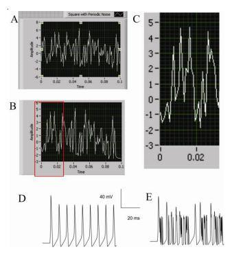
Figure 10: A represent input excitation with Periodic random noise, B the noisy output; C is zoomed output; D shows mathematical simulations of membrane potential recordings without noise; E shows mathematical simulations of membrane potential recordings with noise.
