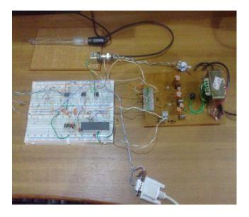
Fig. 7. Hardware implementation of the pH monitoring node
