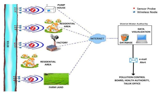
Fig. 1. Proposed Architecture of the River Water Quality Monitoring System
