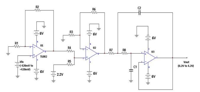
Fig. 4. Signal conditioning circuit
