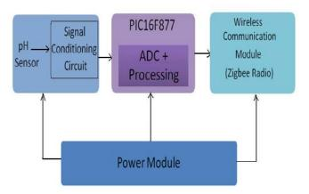
Fig. 3. Wireless Sensor Node for pH monitoring
