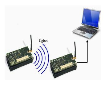
Fig. 5. Wireless transmission of data using MicaZ mote
