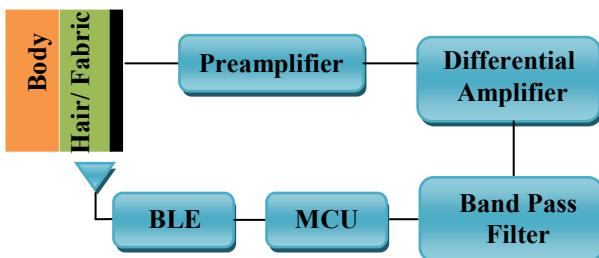
Figure 2. Acquisition system for EOG, EMG and EEG
