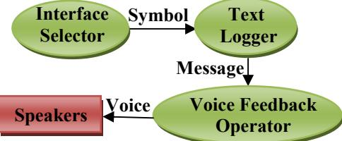
Figure 13. Block diagram of text to speech interface
