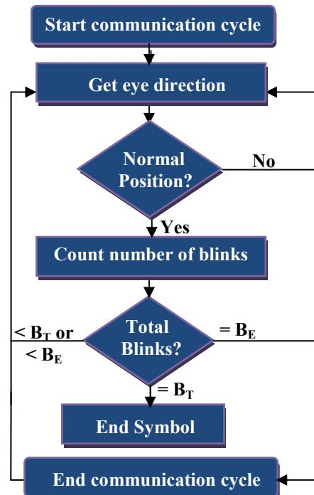
Figure 4. Flow chart of the communication cycle
