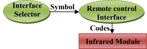
Figure 14. Block diagram of remote control interface
