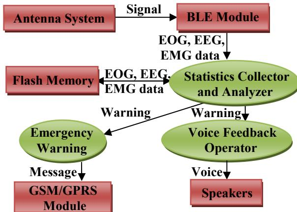
Figure 12. Block diagram of vital statistics collection and analysis
