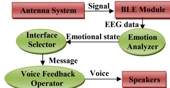
Figure 15. Block diagram of emotion interface
