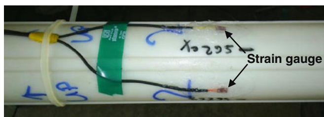
Fig. 8 Strain gauges fixed on an inclinometer casing
