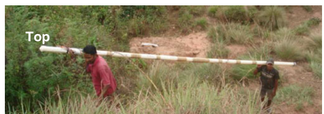
Fig. 9 Strain gauges on an inclinometer casing—ready for installation
