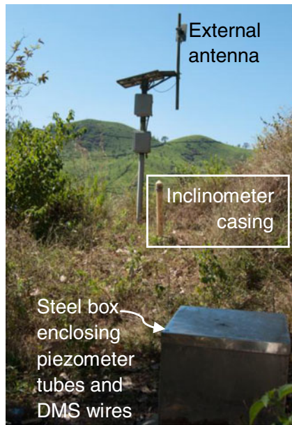
Fig. 14 L_3 after the deployment of the sensors and the wireless sensor network. Refer to Fig. 15 for additional components
