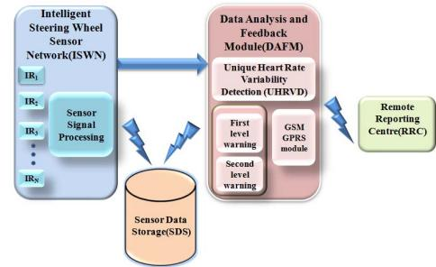
Fig. 1. ISWN detection system
