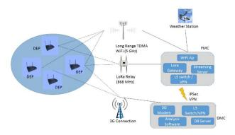
Fig 2.System Architecture
