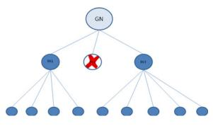
Figure 5: Balanced Two Level Tree WSN after IN Failure and Reorganization
