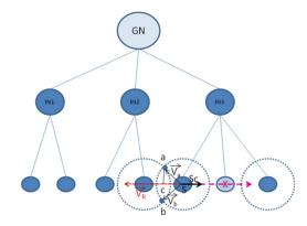
Figure 2: Progressive Two Level Tree WSN before SN Failure
