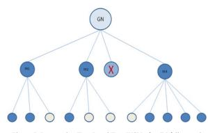
Figure 7: Progressive Two Level Tree WSN after IN failure and reorganization
