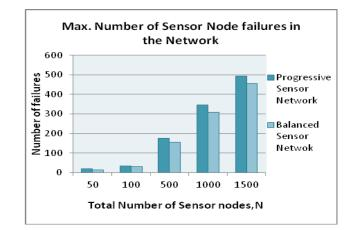
Figure 10: Maximum possible SN Failures in Balanced and Progressive Two Level Tree WSN
