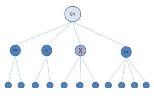
Figure 6: Progressive Two Level Tree WSN before IN Failure
