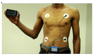
Fig. 3. A patient wearing the Amrita Spandanam ECG sensor device (as a belt). The four body electrodes are connected to the device. The smartphone in the patient's hand shows the live ECG stream as sent from the sensor.
