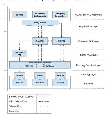
Fig. 1. System Architecture for remote health care service delivery using sensors, IoT devices, cloud and heterogeneous ad hoc networks. Various stakeholder are also shown in this figure.
