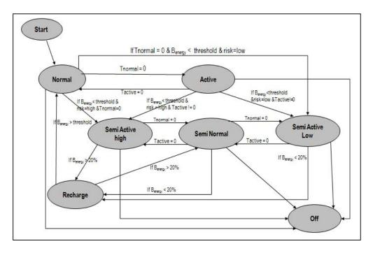
Figure 2. State Transition Diagram for Energy Optimization Algorithm
