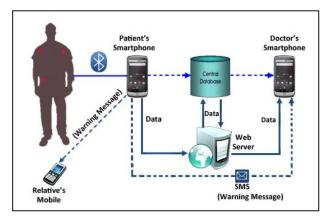
Figure 1. System Architecture
