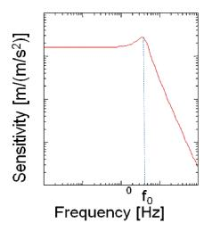
Figure 2. Graph showing the relationship between the geophone sensitivity and frequency of operation. Note the fall in sensitivity after resonant frequency  $(f_0)$ .
