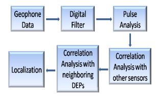
Figure. 5 Shows the pseudo code for the Signal Processing Algorithm for localization
