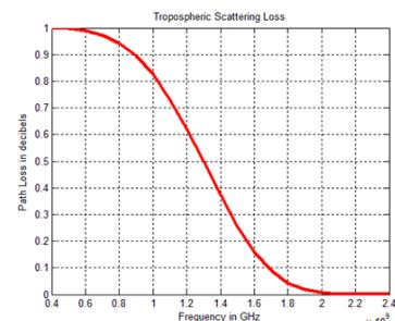
Fig. 4. Tropospheric Scattering Loss
