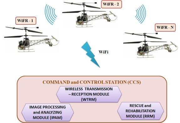
Fig. 2. Architecture of the Real Time Adhoc Networked C- VIEw System
