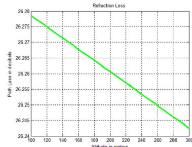
Fig. 3. Tropospheric Refraction Loss
