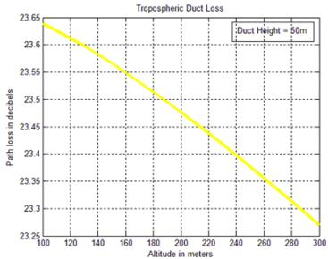
Fig. 5. Tropospheric Ducting Loss
