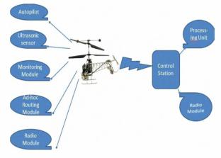
Fig1. Detailed Architecture considering single network element
