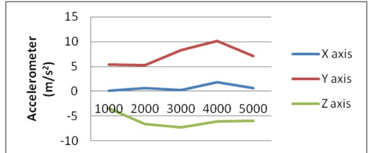
Figure 3. Accelerometer values for fall. X axis indicates time in ms and y-axis indicates accelerometer in  $m/s^2$
