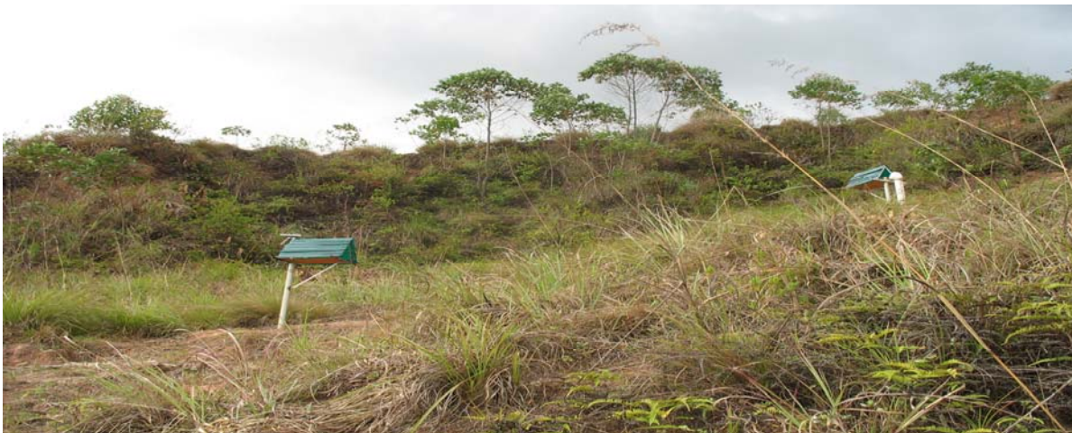
Figure 2: Field deployment of one sensor column and one relay node
